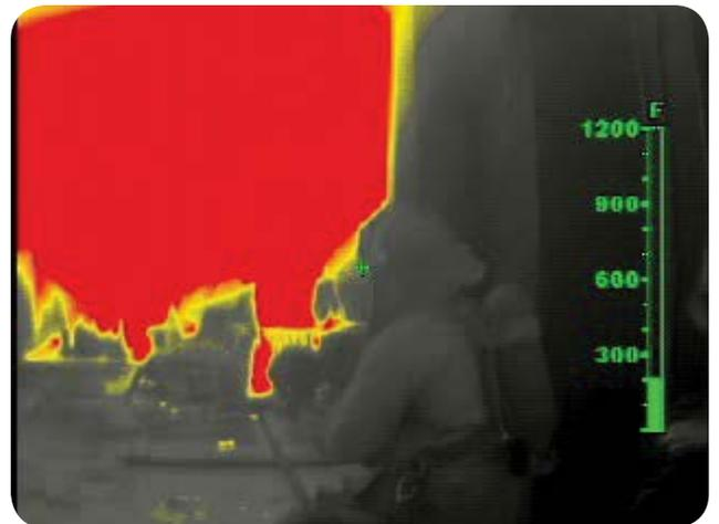
If the TI has a colorization system, then the saturation will be indicated by the "hottest" color (normally red).
