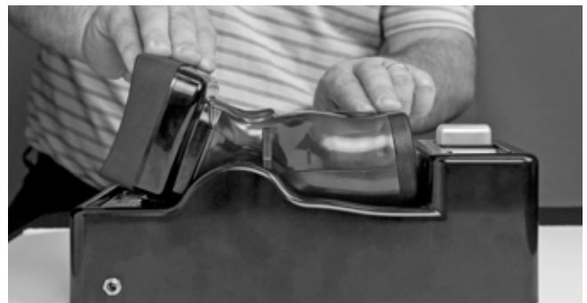
Thermal imager sitting in Powerhouse incorrectly.
