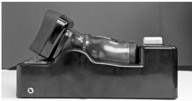
Thermal imager sitting in Powerhouse correctly.
