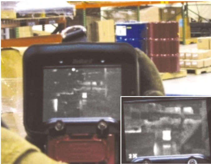
Zoom in on distant objects when getting closer is unsafe or impractical.
