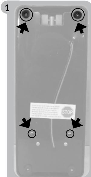
1 Remove four (4) screws from back of Eclipse Powerhouse.
