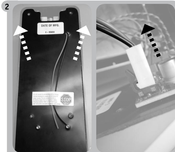
2 Carefully lift back plate (be sure not to rip any wires out). Unplug one connection from board.
